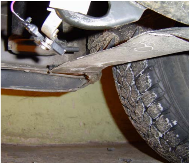
Fig. 3. Transducer placement under the car
