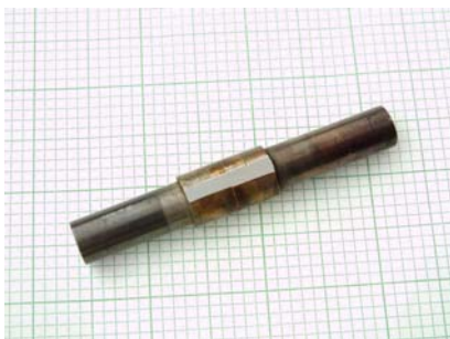
Fig. 7. The bonded stainless steel rods
