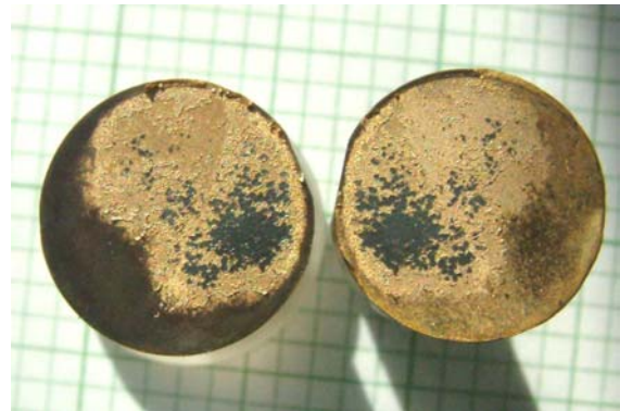
Fig. 9. View of the broken bond after the tensile tests
