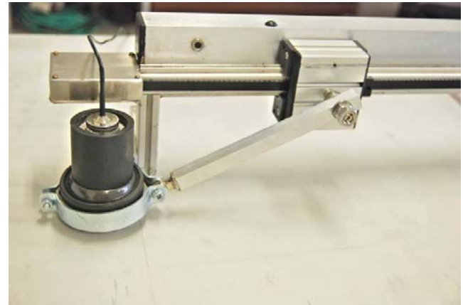
Fig. 4. The photo of the experimental set-up for testing of the wind turbine blade using planar 400 kHz transducer
