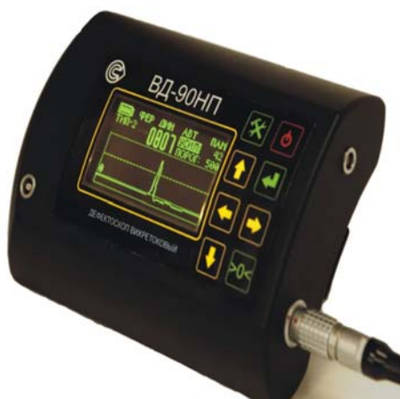
Fig. 1. VD-90NP eddy current flaw detector. General view
