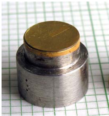
Fig. 3. Stainless steel thick protector with bismuth titanate piezoelement, soldered or thermosonically bonded
